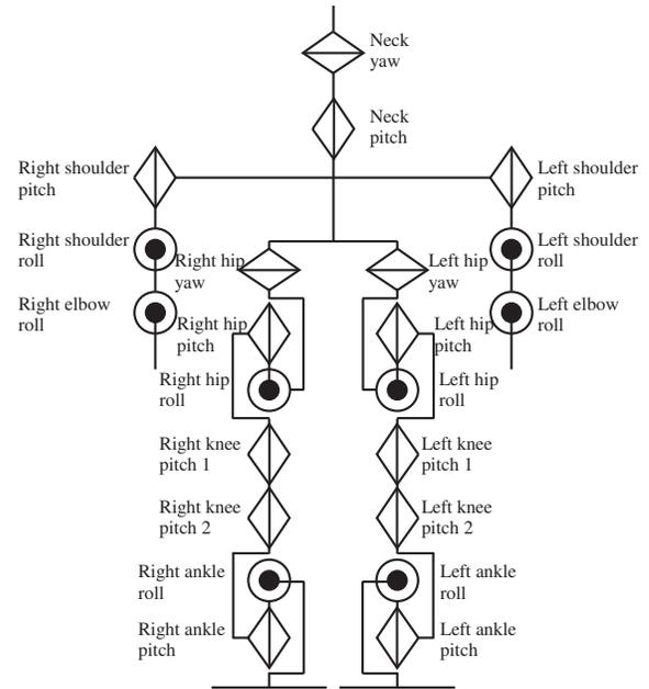
Fig. 2. Degrees of freedom of the developed baby robot.
