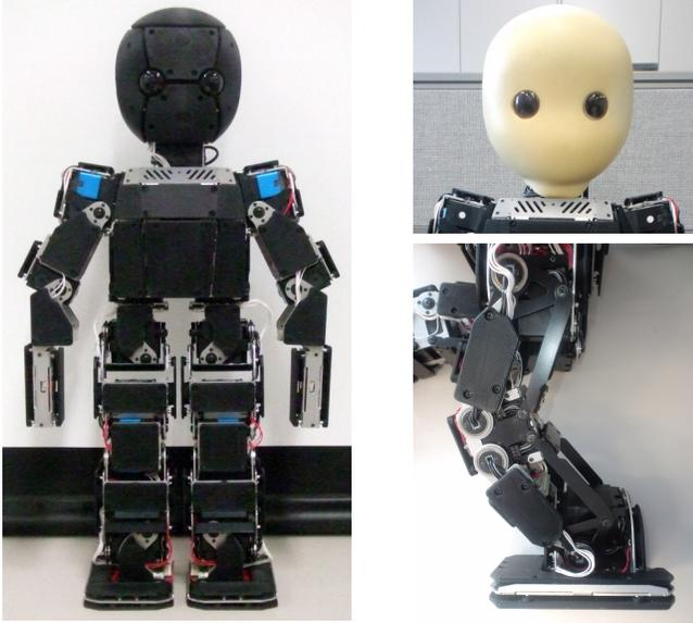
Fig. 1. Photo of the developed baby robot (left), head covered with urethane foam (right top) and detail leg parallel link mechanism (right bottom).
