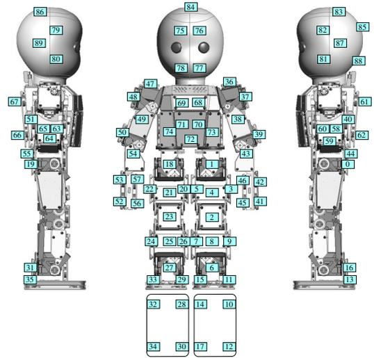
Fig. 7. Arrangement of the touch sensors on the robot body.
