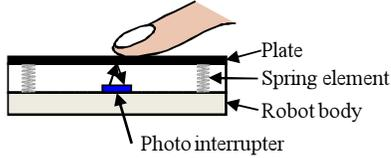
Fig. 6. Schema of our touch sensor.
