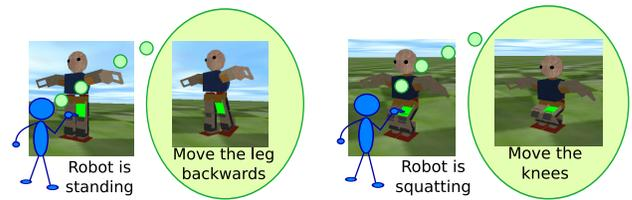
Fig. 8. An example of the context dependence of the touch meaning. The user presses the same sensor, but due to the different robot posture the desired posture modifications (bend the leg and bend the knees, respectively) differs.
