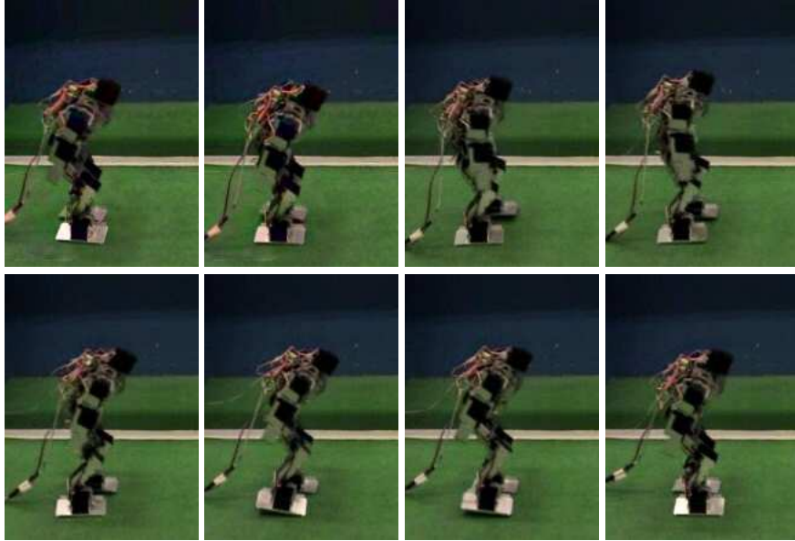
Fig. 5. Snapshots of the walking pattern achieved on the real robot. The time between successive images is 150 ms.
